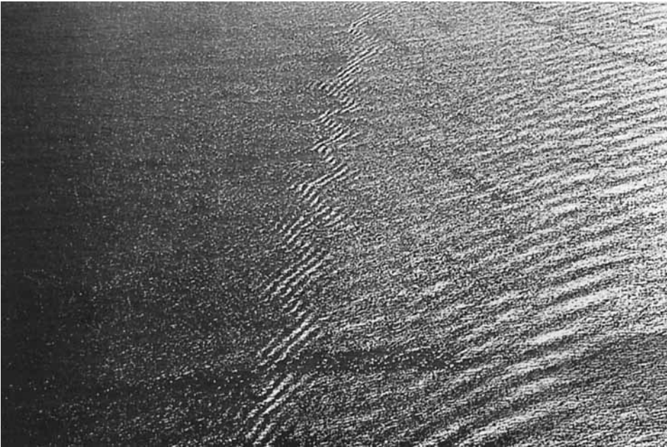
FIGURE 12. Photograph of port side of wake taken during the same aerial survey as figure 2. As discussed in the text, the photograph extends from about 0.7 to 1.9 km aft. The average wavelength of the sinuous fluctuation along the solitary feature is about 0.1 km and the amplitude is roughly \pm 11 m.
